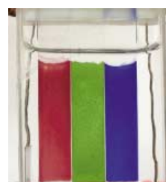
Figure 6. RGB colors obtained from polymeric electrochromic device (PECD): P3MT, PDDTP, and PEDOT were used as red, green, and blue polymers, respectively. The polymer films were held at the same potential of -0.80 V (vs. \text{Ag}/\text{Ag}^+ ) to keep them in their neutral form.
